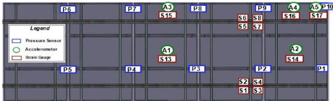
Figure 2. Close-up of the PV panel instrumentation.
